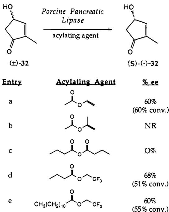
Figure 5. Effect of acylating agent on the resolution of (±)-32.
